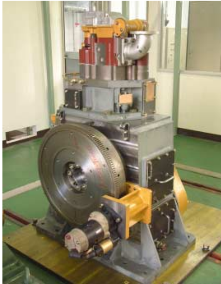
Fig. 4.2.3-1 Assembly of Single Cylinder Test Model
