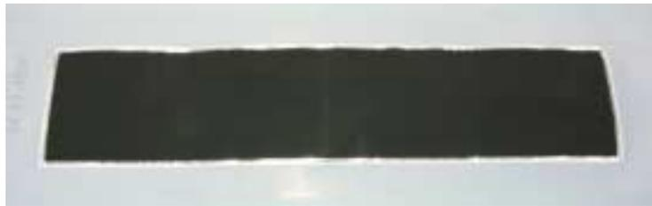
**Fig.8.2.1-3 Membrane electrode assembly (entire view)**
