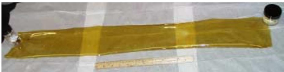
**Fig.8.2.3-1 FSPEEK and PBI A membrane**
