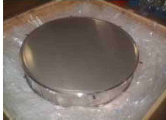
Fig. 9.1.2-2 Panel vacuum type insulation structure specimen
